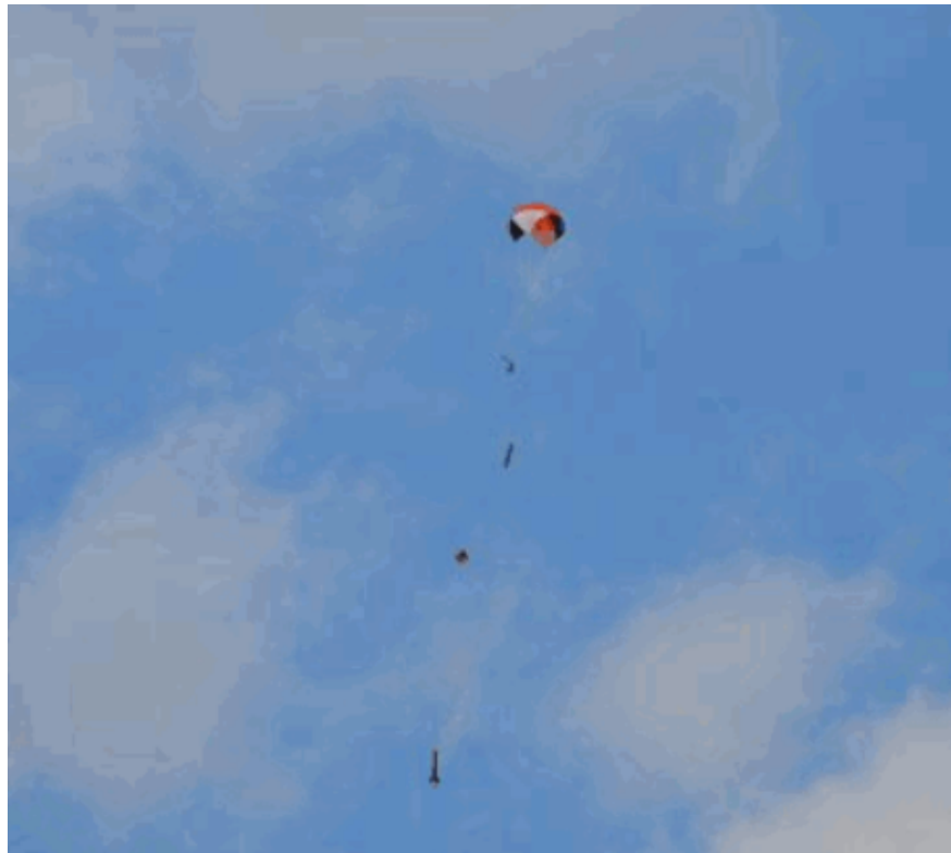
Fig. 31 Full descent of Sabre III under both drogue and main parachutes during Subscale Flight 1 (3/1).
