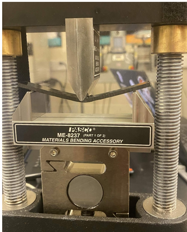
Fig. 35 Three-point bending test of a 1/8" carbon fiber coupon utilizing the PASCO ME-8237 Materials Bending Accessory.
