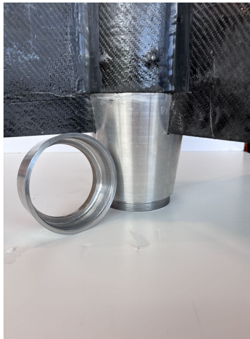
Fig. 5 Sabre III SRAD boat tail.
