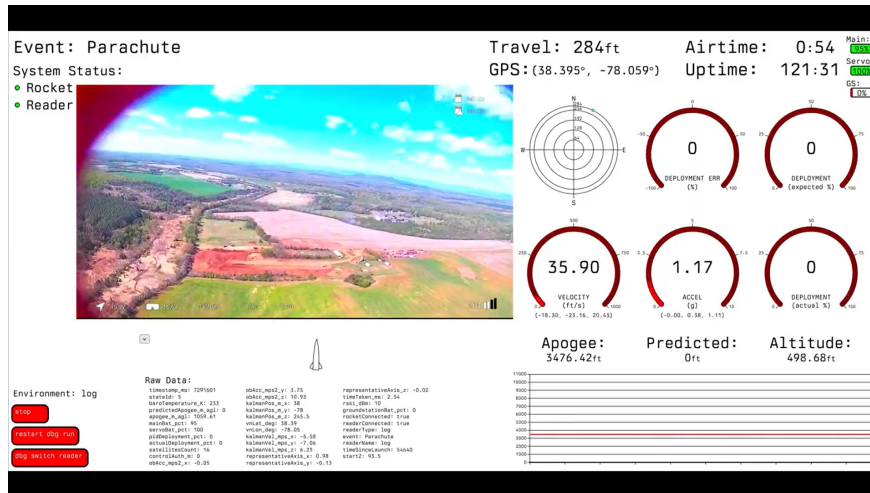
Fig. 33 Onboard live video transmission feed demonstrating the integrated telemetry UI and sensor readings in-flight (4/14).
