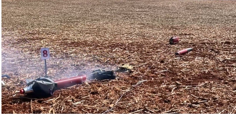
Fig. 28 Successful drogue charge separation (2/28).
